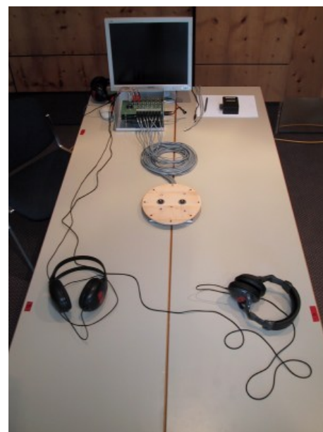
The Smart Microphone Array (SMA): the eight-microphone circular array, and in the back, the DSP-based real time processing unit.
